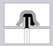
These "U" shaped seals were designed in conjunction with the development of the new generation of pull rings (patent pending).
